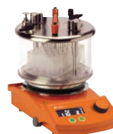
Blowdown base and 24 position MTP
